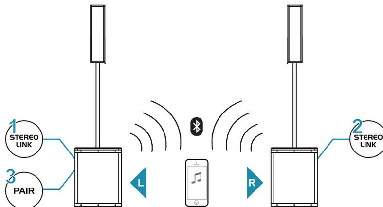
The integrated TWS (True Wireless Stereo) function allows two PA systems to be paired via Bluetooth. The left and right audio channels are played back separately and without delay in stereo via both PA systems.
