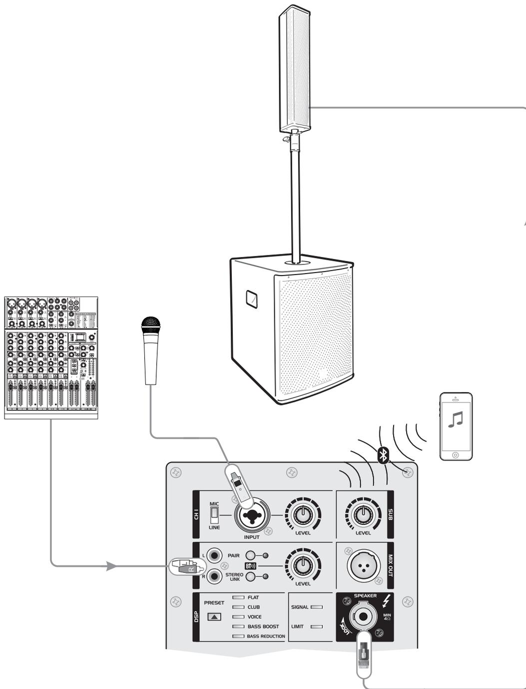
As signal source, microphones and audio units with line level can be connected. To avoid interfering noise, switch off the PA system or set the output controls to minimum prior to connecting and disconnecting equipment. Be sure to use only high-grade cables.
