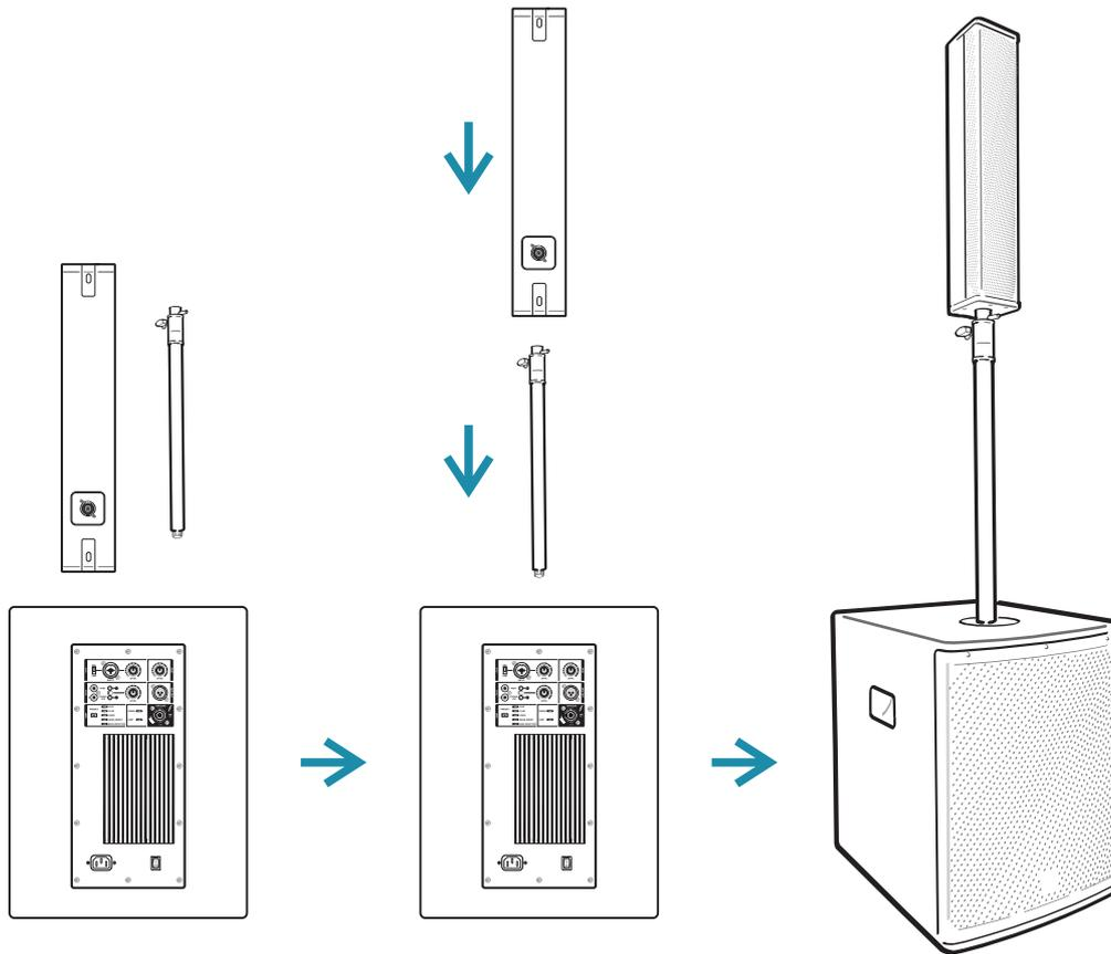
Insert the telescope bar into the flange on the upper side of the subwoofer; then fasten the column module on top. The column's lower speakers should be at ear's height; adjust the telescope bar accordingly. Make sure to insert the locking pin into the telescope bar to secure the height adjustment.
