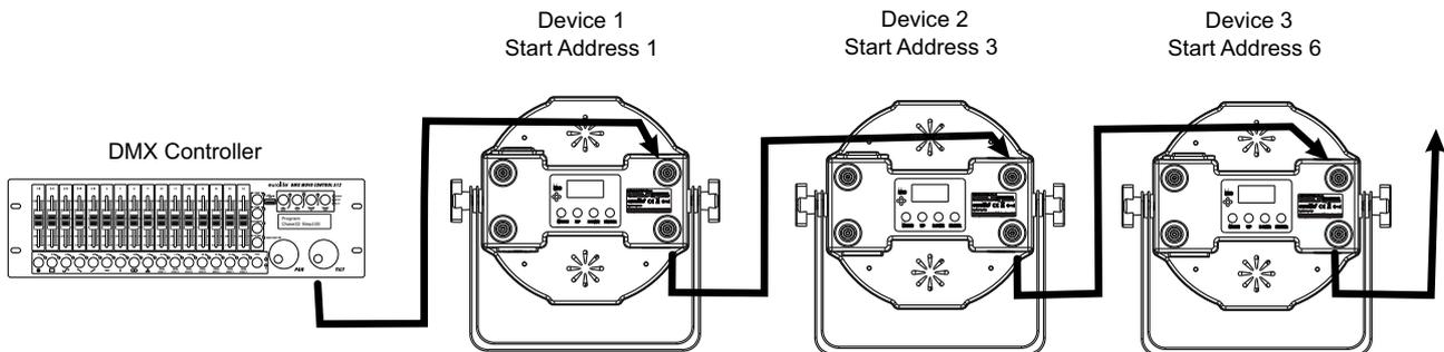
A DMX512 data link is required in order to control the device via DMX. The device provides 3-pin XLR connectors for DMX connection.
