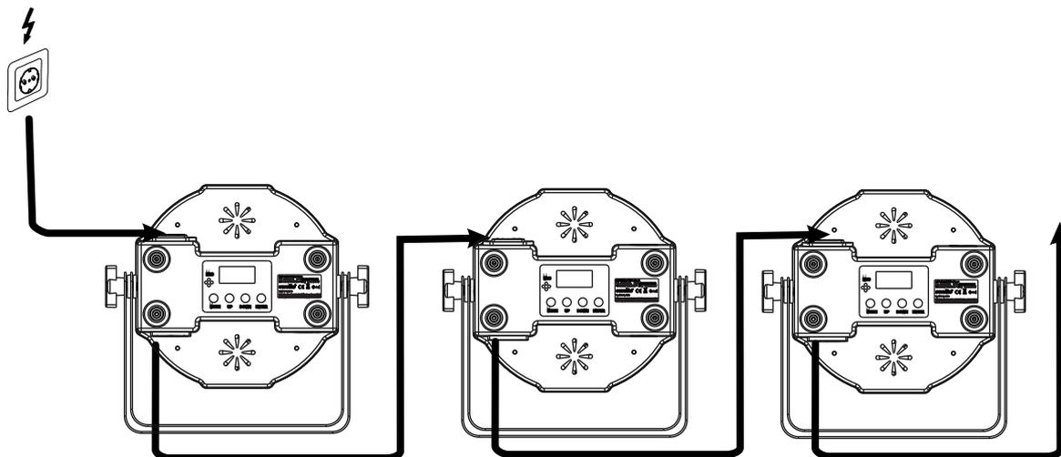
The device uses an auto-range power supply that accepts input voltages between 100 und 240 volts.
