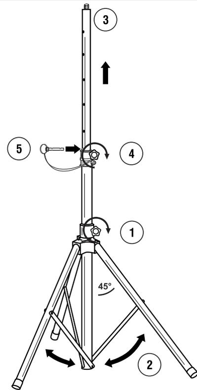
**Pull out the legs** – Loosen the safety screw (1) of the legs. Pull out the legs (2). Lock this position with the safety screw.
