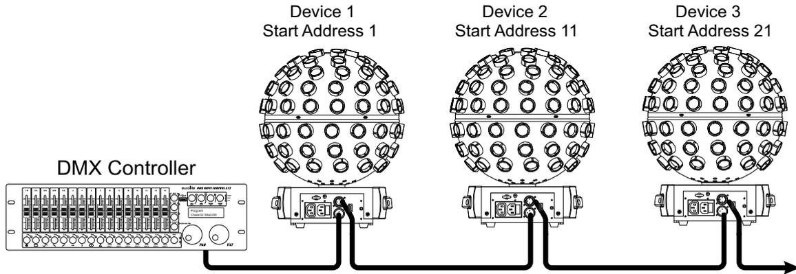
A DMX512 data link is required in order to control the device via DMX. The device provides 3-pin XLR connectors for DMX connection.
