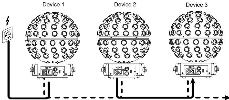
The jack POWER OUT allows for power supply of further devices. To interconnect several devices, connect the jack POWER OUT to the input POWER IN of the next unit until all units are connected. Matching power cables with IEC plugs are available as accessories. In this manner, up to 8 devices can be linked at 230/240 input voltage and up to 4 devices at 110/115 input voltage.
