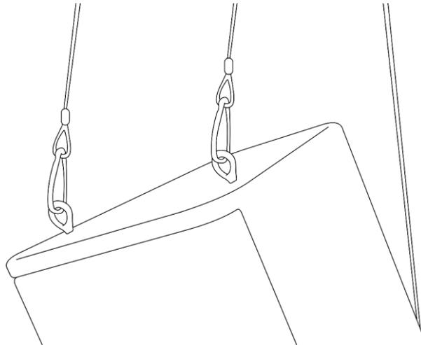
The Pure-15 speaker can be placed on a flat stage floor or be hung from a ceiling by means of the Speaker hanging eye (D8436).
