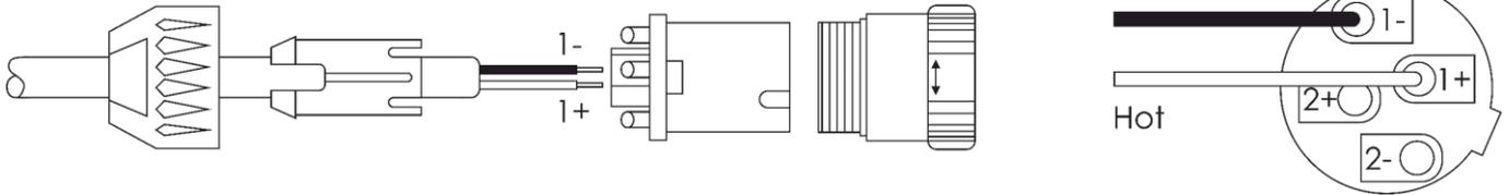
Input is a Speakon connector for connecting a speaker-level signal.
