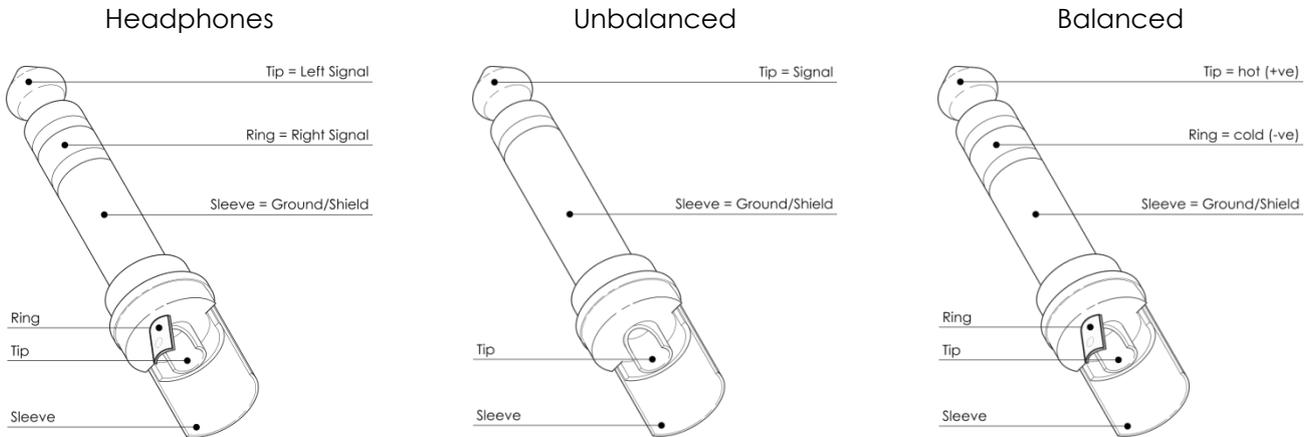
For these applications the unit provides 1/4" TRS and XLR connectors to easily interface with most professional audio devices. Follow the configuration examples below for your particular connection.
