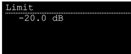
01) Turn the control **(16)** to set the limit. The adjustment range is between -20 dB and 0 dB.
