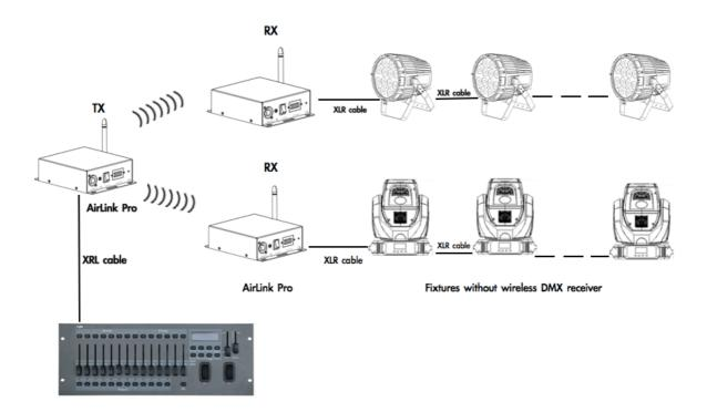
Press the "Pairing" button on the transmitter box, the yellow indicator on the transmitter and receiver box will start to flash at the same time. After a few seconds the wireless DMX indicator will stay On, this means pairing succeeds. Now you can control your fixtures with your lighting desk.
