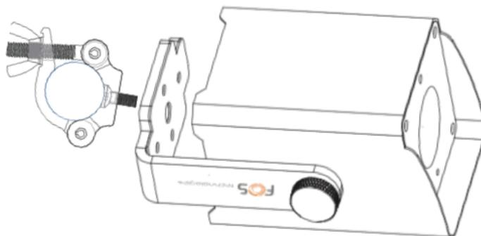
When install the fixture to crossbar or truss, always use an extra safety cord (not supplied with the fixture). Users also need to make sure the crossbar is stable or not moving, and can support a weight of 37 kg (fixture net weight 3.7kg).
