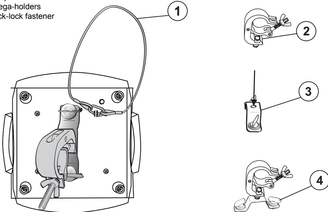
The device may be placed on the floor or fastened to a truss or similar rigging structure. The device must never be fixed swinging freely in the room.
