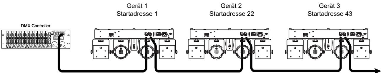
A DMX512 data link is required in order to control the device via DMX. The device provides 3-pin XLR connectors for DMX connection.
