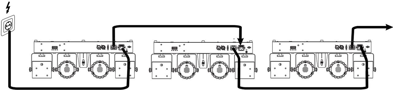
The device uses an auto-range power supply that accepts input voltages between 100 und 240 volts.
