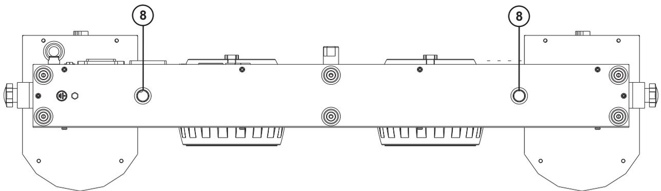
(8) Thread for truss clamp
