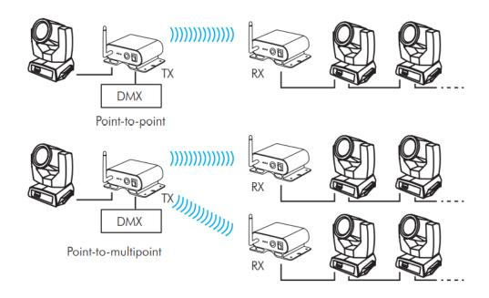
One Transmitter supports one Universe (512 channels) and it can work with the Receivers in Point to Point or Point to Multipoint network types.
