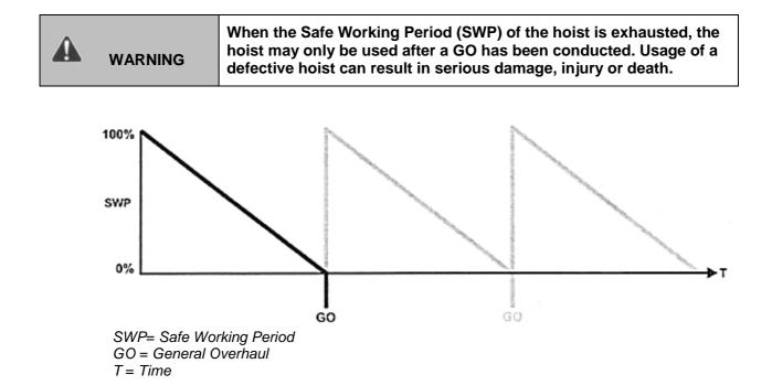
Once the SWP% of the hoisting machinery reaches zero, the hoisting machinery has exhausted its theoretical lifetime. The probability of a defect in the product is therefore higher and operating safety is jeopardized. At the end of the SWP, a thorough General Overhaul (GO) must be conducted. Afterwards the product will then be assigned a new SWP, provided that it is safe to continue operation. At the start of each period the SWP is 100% and, at the end, the SWP is 0%.
