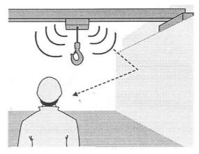
Hoists generate some audible noise during operation. The total noise level experienced in the operating area is a combination of the individual noise sources around the operator. The main sources of noise from the hoist arise from its components, vibrating structures and reflective surfaces.
