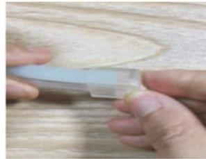
Attach the end cap onto the end of the tube to ensure it is waterproof.
