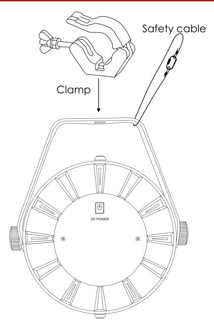
The Bumper Strobe can be placed on a flat stage floor or mounted to any kind of truss with a clamp.
