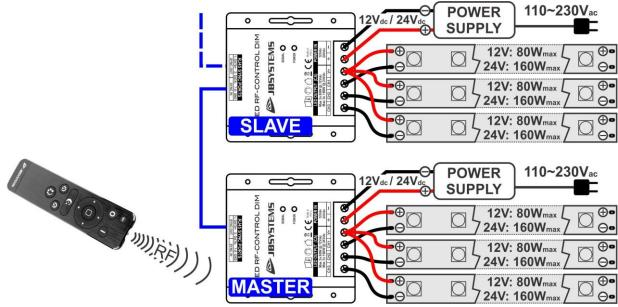
**Remark:** The master (controlled by the RF-remote) is the one where the SYNC IN port is empty.
