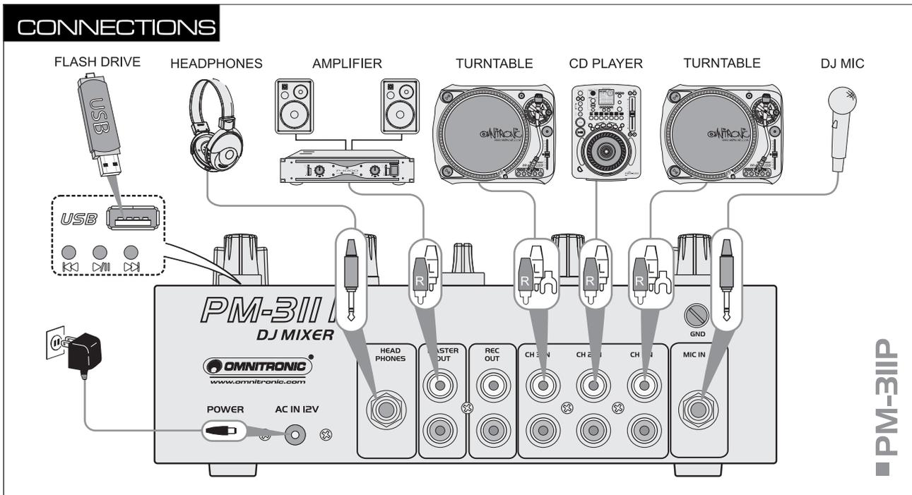
Switch off the mixer prior to connecting any units or to changing any existing connections.
